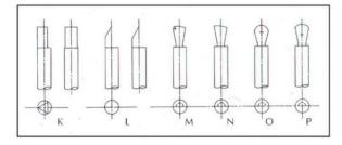
For grinding HSS High Speed Steel and Carbide engraving cutters. Single lip and multiple lip cutters of various shapes such as radius, negative tapered and angled cutters. A universal index head is provided with 24 positions so that any particular angle or shape can be obtained with free 360° or 180° rotation.
